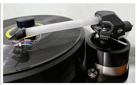
navector XV-1S and my Zu Audio modified Denon DL-103, which is known (or widely believed) to work best in a heavyweight arm. (At less than one-20th the price of the arm, the Zu Denon is admittedly an unlikely pairing.) Mounted on the Safir, none of the three cartridges showed any signs of (di)stress or woofer pumping.
