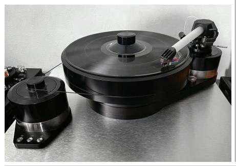
for the horizontal. This hybrid approach gives you the advantages of a zero-clearance design like a unipivot combined with the stability of a traditional gimbal.
