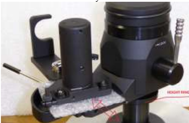
Fig.2A. Pull out fixing foam on the horizontal bearing assembly
