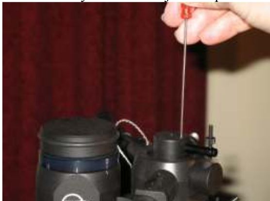
Fig.10 Fixing vertical damping holder
