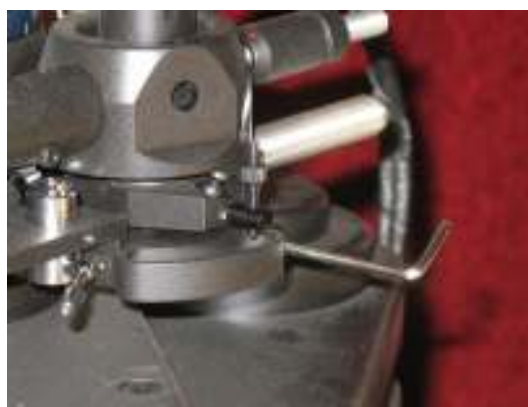
Fig.12 Removing horizontal trough
